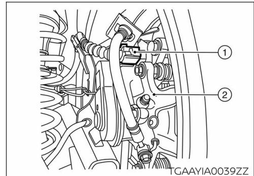
2. Remove the parking brake actuator ( **2** ) from the rear brake caliper assembly ( **1** ).
