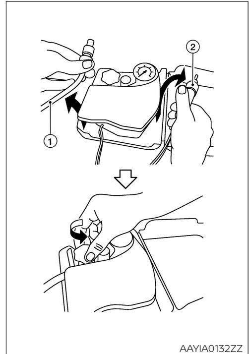
3. Remove the cap from the tire sealant bottle and screw the bottle clockwise onto the bottle holder. Leave the bottle seal intact. Screwing the bottle onto the bottle holder will pierce the seal of the bottle.
