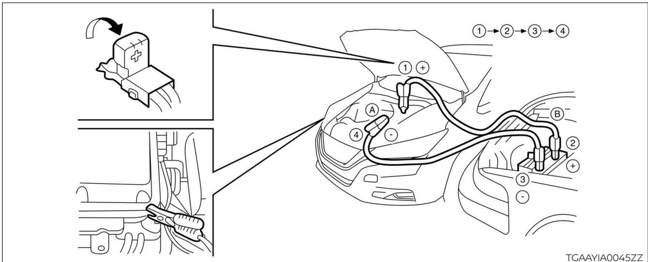
1. If the booster battery is in another vehicle ( **B** ), position the two vehicles ( **A** and **B** ) to bring their 12-volt batteries into close proximity to each other.
