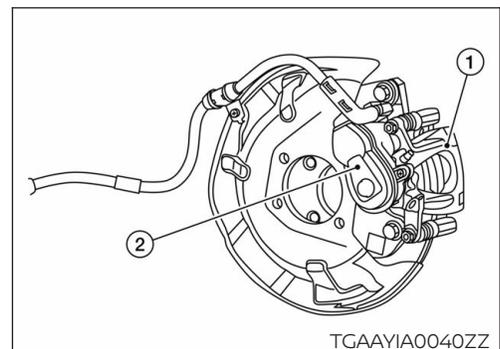
3. Rotate the rear brake caliper assembly ( **1** ) spindle part ( **A** ) clockwise to release the parking brake.
