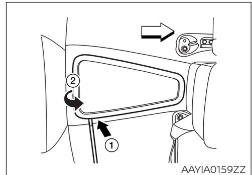
5. Remove the 10 mm access cover bolts ( **1** ) and remove the cover ( **2** ).
