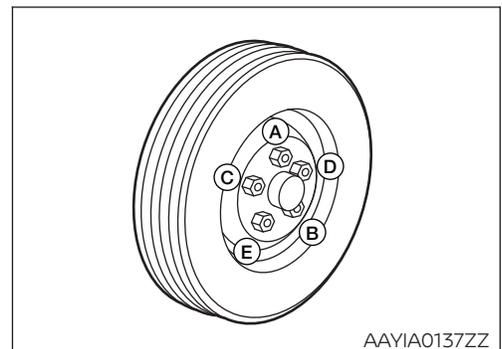
5. Securely torque the wheel nuts in an alternating pattern to 83 ft-lbs (113 Nm).
