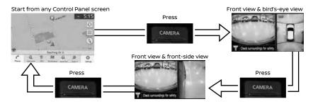
■ When the vehicle is in the R (REVERSE) position and the CAMERA button 1 is pressed, the following views will display in order:
