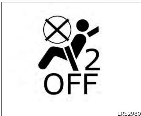
Front passenger air bag and status light
