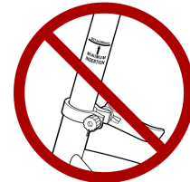
Seatpost out TOO FAR The minimum insertion point on the seatpost must be inserted into the seat tube.
