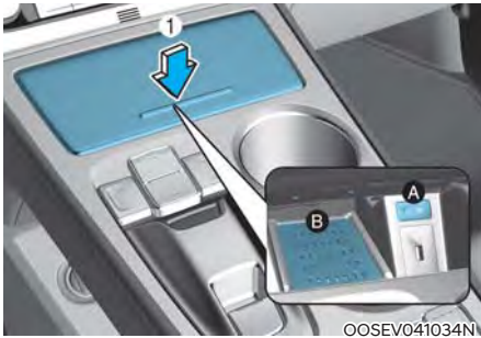
[A] : Indicator light, [B] : Charging pad
