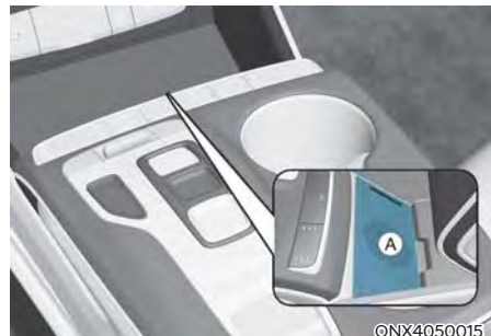
[A] : Wireless Charging Pad (In-vehicle Authentication Pad)
