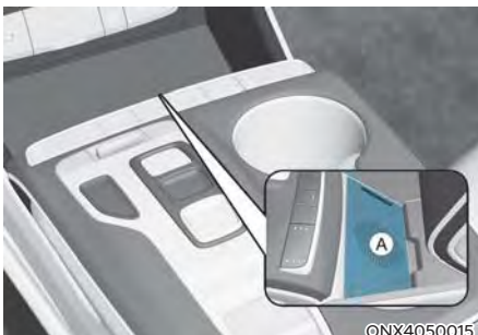
[A] : Wireless Charging Pad (In-vehicle Authentication Pad)
