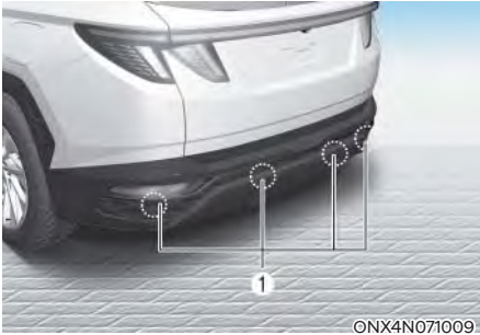
[1] : Rear ultrasonic sensors
